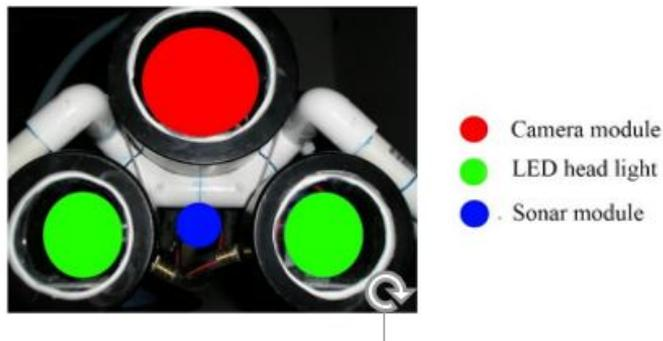
**Figure 4.** Components of the Under Water ROV
