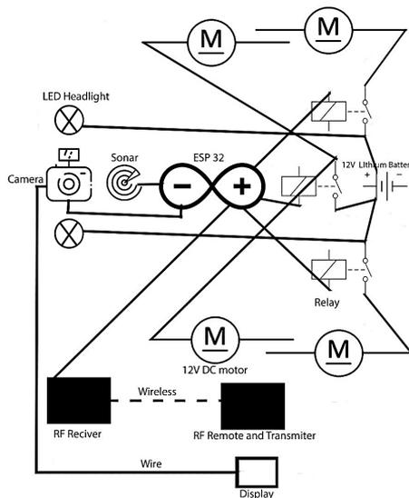
**Figure 2.** Circuit Diagram of the Under Water ROV (The symbol M indicates the motors used)
