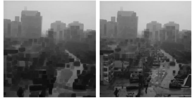
Fig.4. Effectiveness of the proposed scene-specific dark channel. (a) Dark channel of DCP [12] approach. (b) Proposed scene-specific dark channel.
